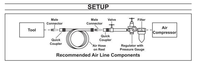
For best service you should incorporate a regulator and inline filter on the compressor end of the hose, as shown in the diagram above. Hoses, couplers, regulators, and filters are all available at Harbor Freight Tools.
